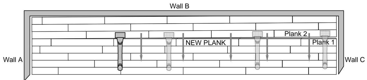
**10.** Lock together the short sides of the replaced plank, continuing along the full row until all short sides are re-engaged. Next, re-engage all the long sides, starting by the planks nearest to Wall A. The repair is complete when all joints are re-engaged.
