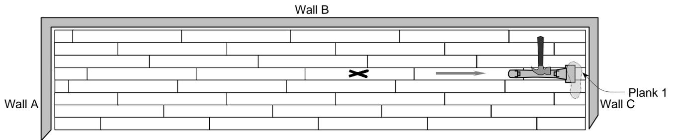
5. Adhere the Bulldog to the plank closest to Wall "C" (plank 1), on the row with the marked plank, by placing one foot on top of the hinged section, and tap the tool so that the plank slides towards the wall until it unlocks from the rest of the row. To disengage the tool from the plank, raise the tool on the hinge and, carefully, rock it from side to side.
